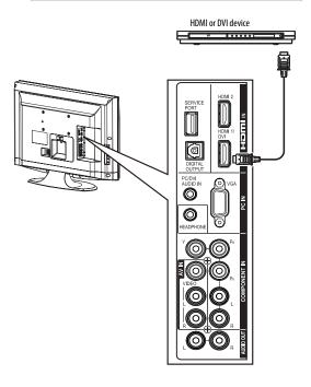
3 If you are connecting a DVI device, connect an audio cable with stereo mini plug (not provided) to the PC/DVI AUDIO IN jack on the back of your TV and to the AUDIO OUT jack on the DVI device.
